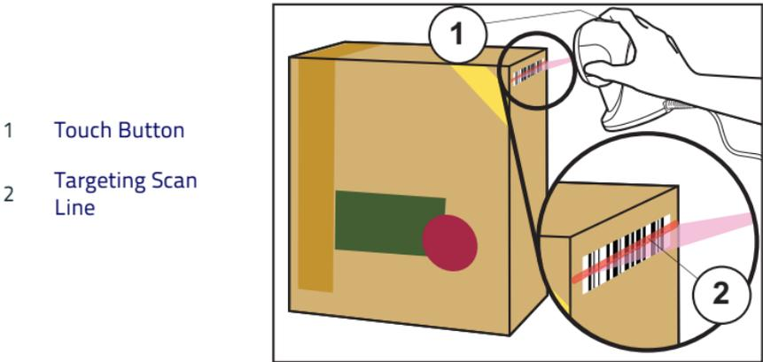
3. Center the single scan line on the bar code to maximize reading capability. Small bar code labels should be moved closer to the scan window, while larger labels need to be held at a further distance.
