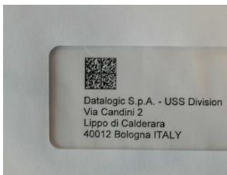
Figure 14 - Address Coded in Data Matrix Symbology for Automated Mail Processing
