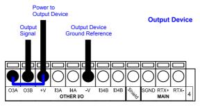
Figure 41 - Output 3 Using DS8100A Power
