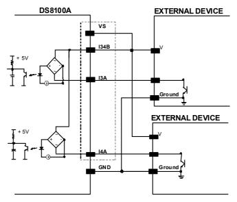
Figure 56 - I3/I4 NPN Input Command using Scanner Power
