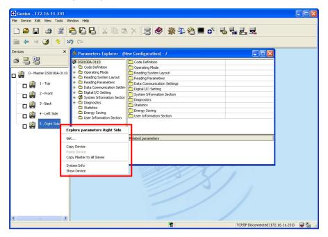
These shortcuts are made only in Genius<sup>™</sup> and require sending the configurations to the scanners to be saved.
