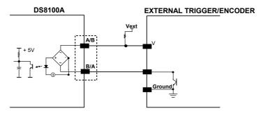
Figure 55 - NPN Command Input Connection Using External Power
