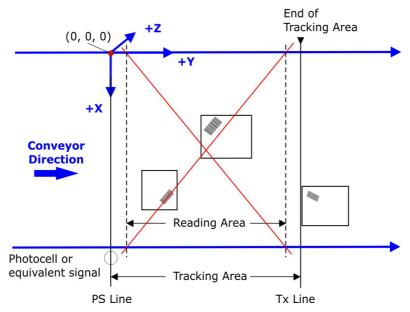
Figure 94 - PackTrack™ System Layout
