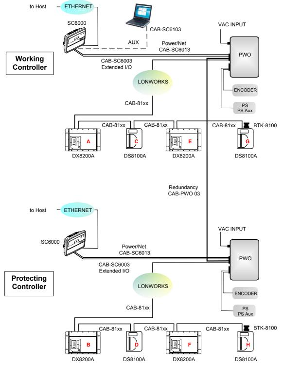
Figure 77 - Redundant Reading Station Layout with DX8200A and DS8100A Scanners
