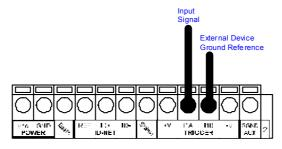
Figure 26 - PNP External Trigger/PS Using External Power (i.e. PLC signal)
