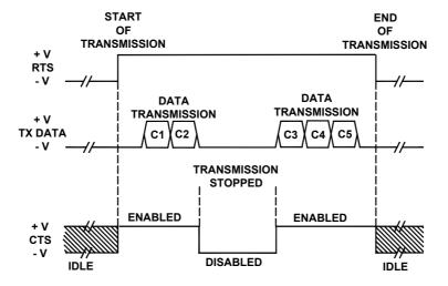
Figure 46 - RS232 Control Signals
