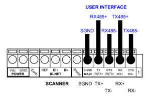
Figure 18 - RS485 Full-duplex Connections
