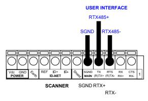
Figure 20 - RS485 Half-duplex Connections
