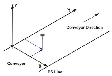
Figure 95 - PackTrack™ Reference System
