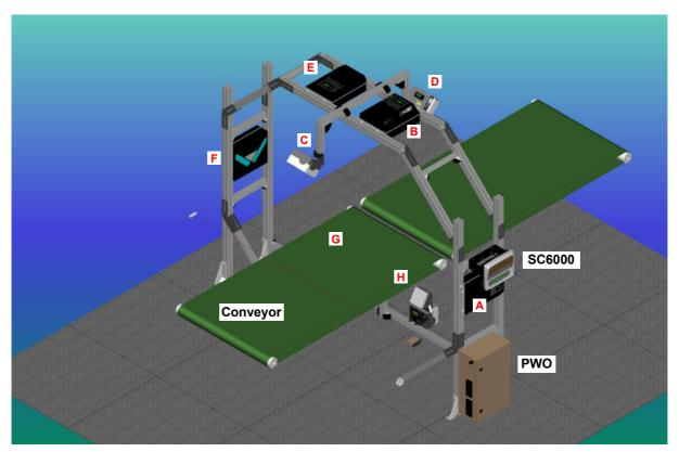
Figure 76 – Example Large Synchronized Network Reading Station
