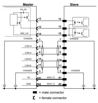
Figure 63 - DS8100A Master/Slave Lonworks Connection
