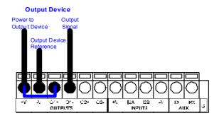
Figure 36 - Open Emitter Output Using DS8100A Power
