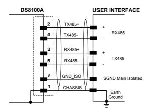
Figure 47 - RS485 Full-Duplex Interface Connections
