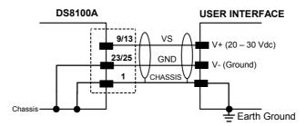
Figure 44 – Power Supply Using the 26-pin Connector
