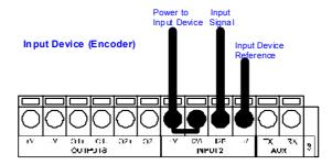
Figure 29 - Encoder NPN Using DS8100A Power
