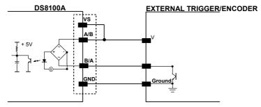
Figure 53 - NPN Command Input Connection Using Scanner Power
