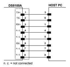
Figure 72 – Inverted Cable
