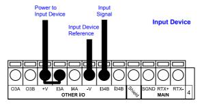
Figure 33 - NPN Input 3 - 4 Using DS8100A Power
