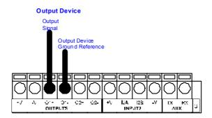
Figure 39 - Open Collector Output Using External Power
