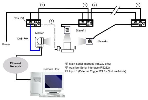
Figure 109 - RS232 Master/Slave for DS8100A Ethernet Models
