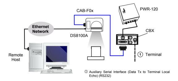
Figure 104 - Point-to-Point for Ethernet Models
