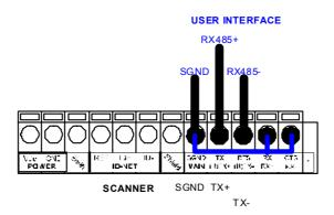
Figure 19 - RS485 Full-duplex Connections using Only TX Signals
