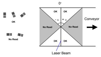
Figure 93 – Reading Zones with  $\alpha$  Max
