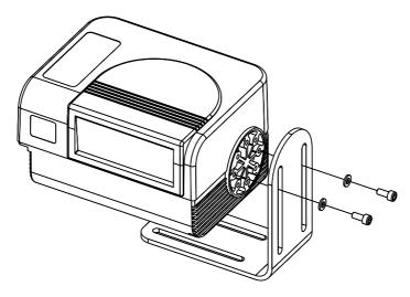
Figure 9 - Mounting the ST-163 Mounting Bracket
