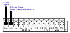
Figure 42 - Ouput 3 Using External Power
