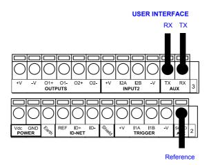
Figure 23 - RS232 Auxiliary Interface Connections
