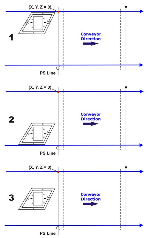
3. The Absolute X coordinate requires placing the barcode label **centered** onto the physical X position (X Offset) on the conveyor (previously set in the dialog box), you have 2 minutes to read the code before the procedure ends automatically.
