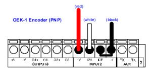
Figure 28 - OEK-1 Encoder PNP Using DS8100A Power
