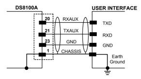
Figure 51 - RS232 Auxiliary Interface Connections
