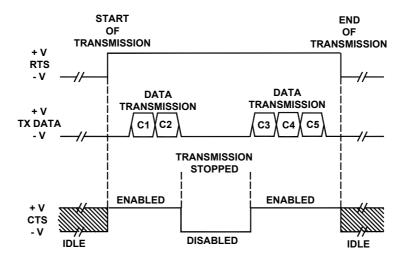
Figure 17 - RS232 Control Signals
