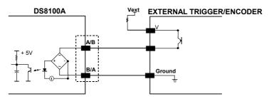
Figure 54 - PNP Command Input Connection Using External Power
