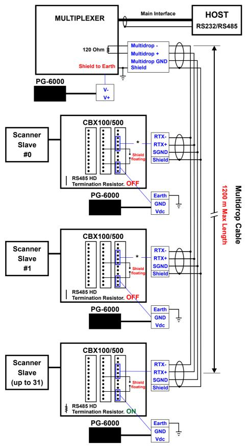
Figure 21 - DS8100A Multidrop Connection to a Multiplexer
