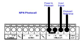
Figure 25 - NPN External Trigger/PS Using DS8100A Power
