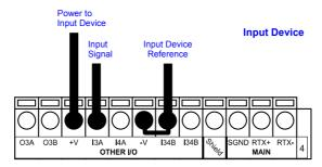
Figure 32 - PNP Input 3 - 4 Using DS8100A Power
