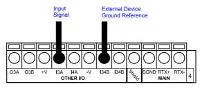
Figure 34 - PNP Input 3 - 4 Using External Power (i.e. PLC signal)
