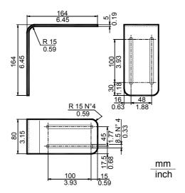
Figure 7- ST-163 Mounting Bracket Overall Dimensions
