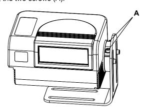
Figure 11 - Substituting a Scanner
