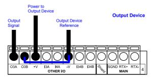
Figure 40 - Output 3 Using DS8100A Power
