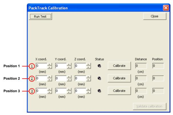
Figure 100 – Performing the PackTrack™ Calibration
