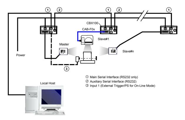
Figure 108 - RS232 Master/Slave for DS8100A Standard Models
