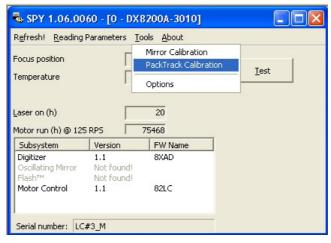
Figure 99 – Selecting PackTrack™ Calibration Option
