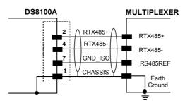
Figure 49 - RS485 Half-Duplex Interface Connections
