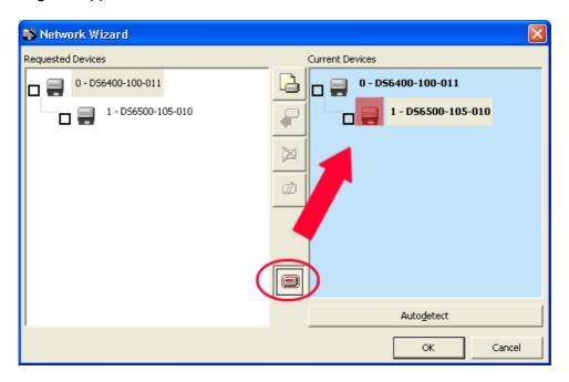
The "Show Device" option is particularly useful after the Net-Autoset procedure or whenever it is necessary to know which address is assigned to a specific slave scanner. Indeed, it activates the following signals which physically indicate the scanner corresponding to the one selected, in particular:
