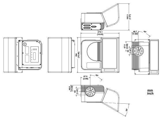
Figure 8 - DS8100A Oscillating Mirror Model Overall Dimensions
