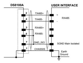
Figure 48 - RS485 Full-duplex Connections using Only TX Signals
