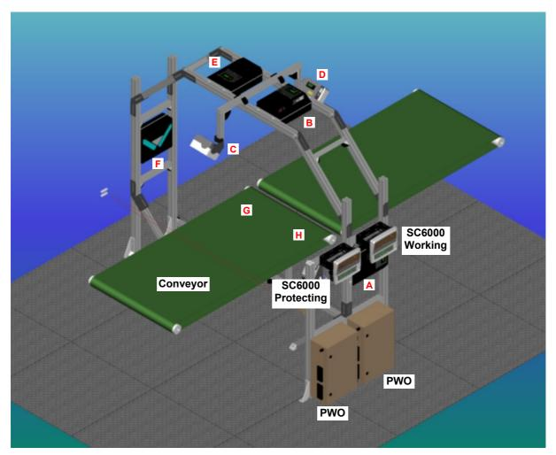
Figure 78 – Example Redundant Reading Station
