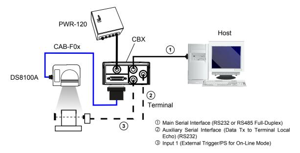
Figure 103 - Point-to-Point for Standard Models
