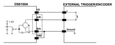
Figure 52 - PNP Command Input Connection Using Scanner Power
