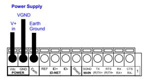
Figure 15 - Power Supply Connections
