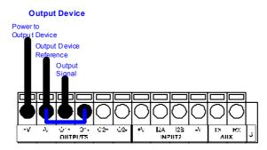
Figure 37 - Open Collector Output Using DS8100A Power
