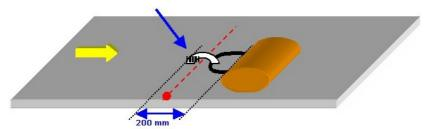
To correct this, set the following Operating Modes parameters: Minimum Distance Between Packs = 200 mm, Minimum Pack Length = 200 mm, Window Dimension = 200 mm.
