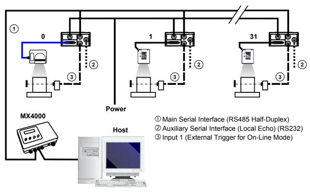
Figure 110 - Multiplexer for DS8100A Standard Models
