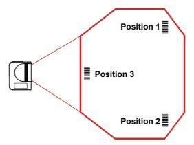
5. Measure the X, Y and Z coordinates relative to the **center** of the code and enter them into the corresponding edit boxes.
