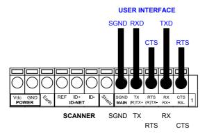
Figure 16 – RS232 Main Interface Connections Using Hardware Handshaking
