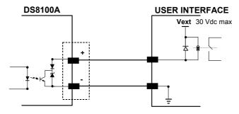
Figure 58 - Output 1 and Output 2 Interface
