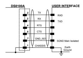
Figure 45 - RS232 Connections
