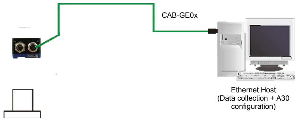
Figure 45 - Standalone Layout to Ethernet Host (Point-to-Point)
