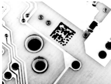
Figure 23 - Data Matrix Code Directly Marked on PCB Surface by Using Laser Etching Technology
