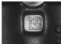
Dot Peening On Scratched Surface
