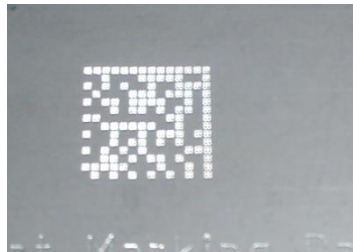
Figure 20 - Dot Peening Marking on Metal Surface with Multi-dot per Code Element
