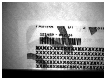
Figure 17 - Overprinted Barcode Readable by Matrix 300N™ also Through the Envelope Window Film
