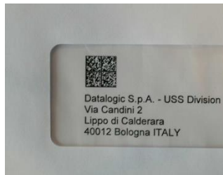
Figure 15 - Address Coded in Data Matrix Symbology for Automated Mail Processing
