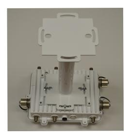
4. With the Access Point positioned so that the gore vent is facing down, attach the extension arm to the Access Point bracket section with two ½ inch bolts and nuts. Tighten bolts to 300 inch pounds (lbf-in).
