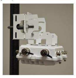
Rotate the Access Point bracket section upward and align the top holes on the sides with the top holes on the angle adapter bracket section. Insert two M6 hex flange screws into the top holes on the angle adapter bracket section.
