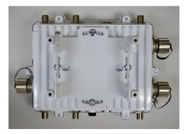
4. Insert two M6 hex flange screws into the bottom holes on the sides of the Access Point bracket section.
